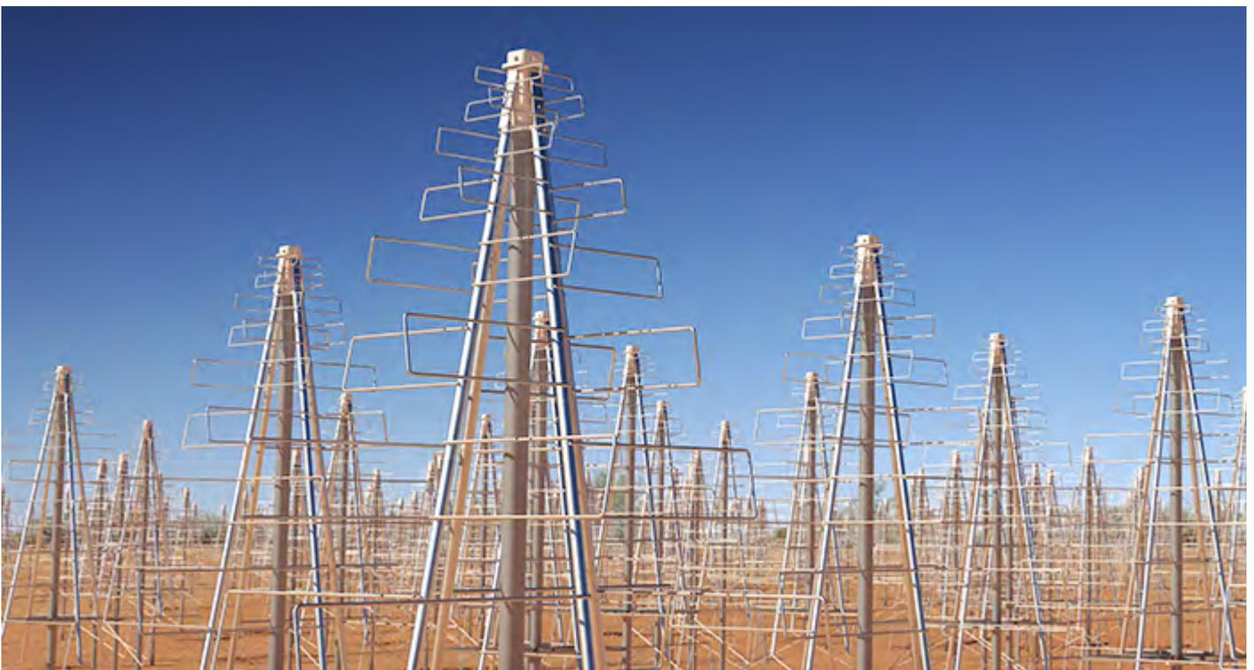
**Above:** A visualisation of the low frequency antenna array to be constructed in Australia, based on development work carried out in the Astrophysics Group. The array will consist of over 100,000 such antennae with a collecting area of 1 square kilometre.
