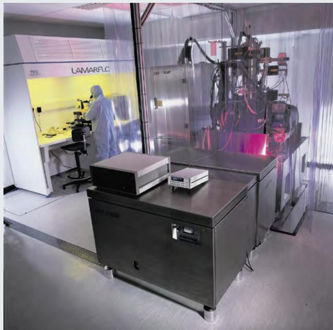
**Above:** Leica VB6 UHR electron beam lithography machine for nanoscale patterning of semiconductor structures.
