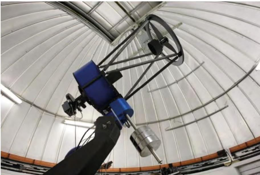
**FIG. 1.** The 60-cm TRAPPIST telescope at the La Silla Observatory in Chile. The acronym stands for TRAnsiting Planets and Planetesimals Small Telescope.<sup>1</sup>
