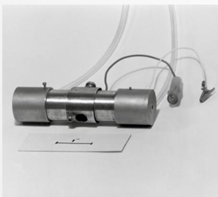
**FIG 2.** The proportional counter used to measure the X-ray spectrum of light elements such as oxygen and carbon.
