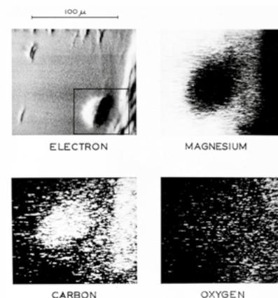
**FIG 4.** Images of a magnesium specimen with a carbon inclusion, previously thought to be an oxide inclusion.
