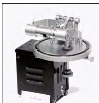
outside the vacuum chamber and these are all functional in the replica. No attempt was made to make the proportional counter an active device. The gas in the counter was argon and had to be continuously maintained at a standard pressure by a flow of the gas through the plastic tubes seen in the photographs.
