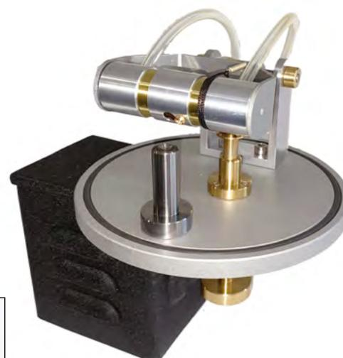
**FIG. 1. The proportional counter used to measure the X-ray spectra of light elements such as carbon. (Above) Replica designed and built by Sean Geraghty. (Inset) A photograph from Dolby's dissertation.**
